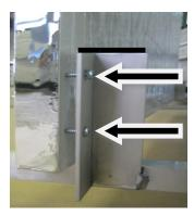
2. Line up the edge of the bracket with the edge of the mirror panel.
